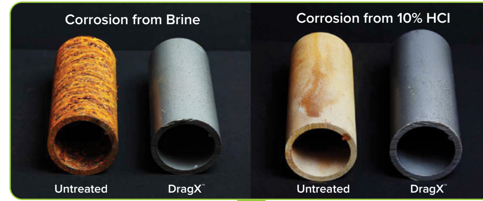
Images comparing untreated and DragX™ treated pipes corroded by brine (left) and 10% HCl (right).
