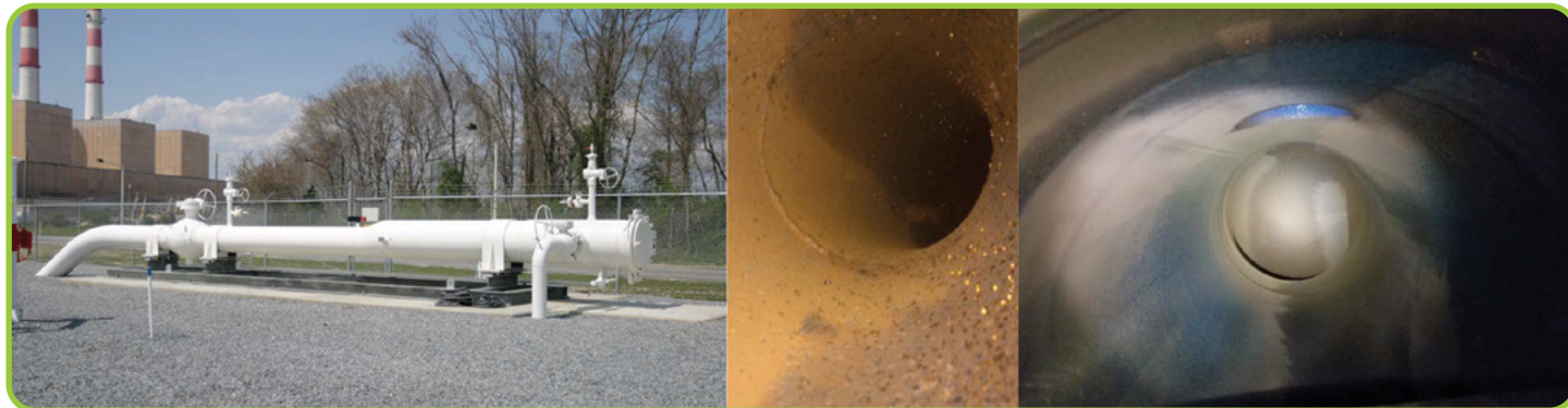
Representative image of test feeder line to simulate pig launcher (left), unprotected section (middle), and DragX™ treated section (right).
