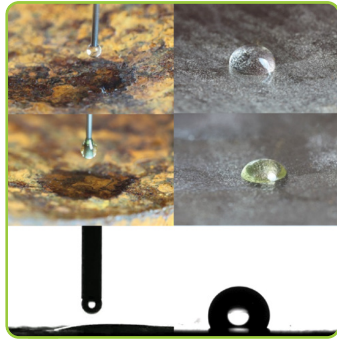
Image of water droplet on untreated pipeline (left) vs DragX™ treated pipeline (right).
