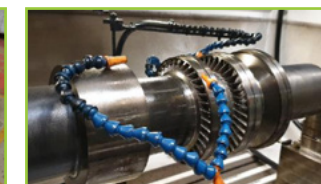
Turbine Rotor EDM First Stage Progress
